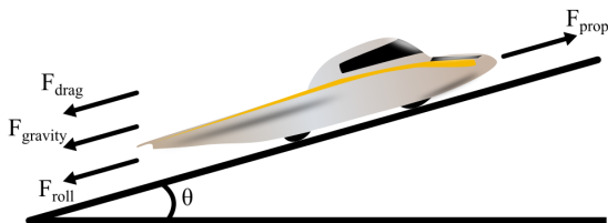
Figure 2.5: Schematics of the forces acting on the solar-powered EV in Paper C.
