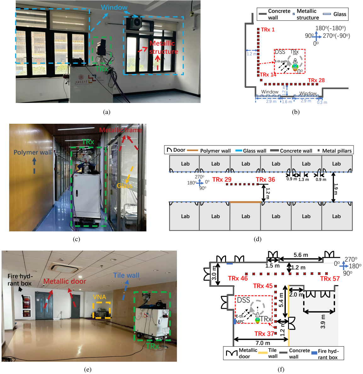
Fig. 1. Diagrams and photos of the measurement scenario for THz monostatic sensing. (a) Real photo in Scenario 1. (b) Diagram of Scenario 1. (c) Real photo in Scenario 2. (d) Diagram of Scenario 2. (e) Real photo in Scenario 3. (f) Diagram of Scenario 3.
