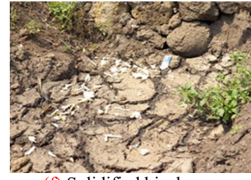
(f) Solidified bioslurry indicating inconsistent feeding.
