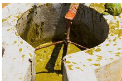
(a) Water and solid feedstock mixing before feeding.
