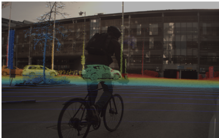
Figure 2.2: Parallax effects in multiview sensor setups (© Zenseact AB). Due to sensor placement, the lidar beam overshoots the pedestrian, making the joint interpretation of objects between camera and lidar ambiguous.
