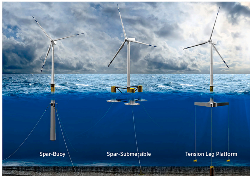
Fig. 6. Design of floating wind turbine foundations [77].
