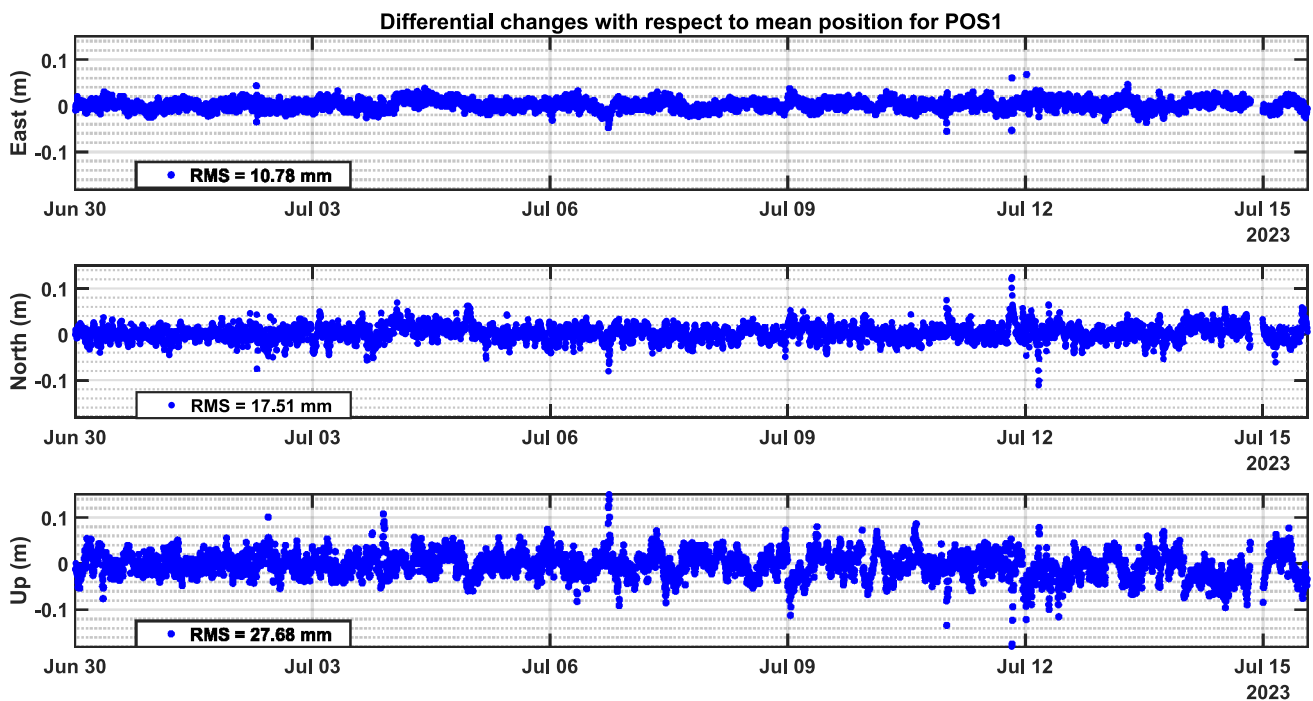
Fig. 10 Time series of relative POS1 east, north and up components in meter with respect to mean position estimates computed using GipsyX PPP processing with GPS, GLONASS and Galileo data
