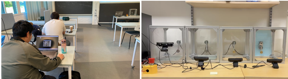
Figure 3: Impressions from pilot study 2 in TRA455 course: instructor with physical access and students with remote access to cloud pendulum hardware during the in-class activity (left), 3 pendulum units connected to the cloud which students can connect to (right)
