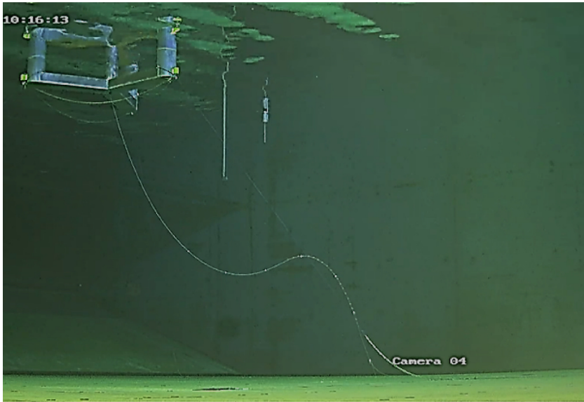
Fig. 14: 1:70 scale testing of the Voltturn US platform, moorings and dynamic cable in the COAST ocean basin (Photo Credit: A. Holcombe)
