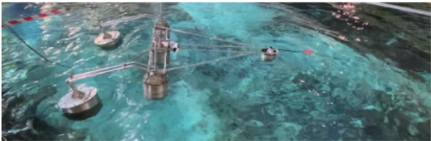
Fig. 26: Aerial photo of WEC with mooring in the wave basin
