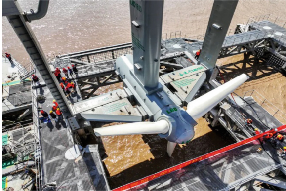
Fig. 31. China's Endeavour tidal stream turbine (source: https://www.seetao.com/details/141111.html )
