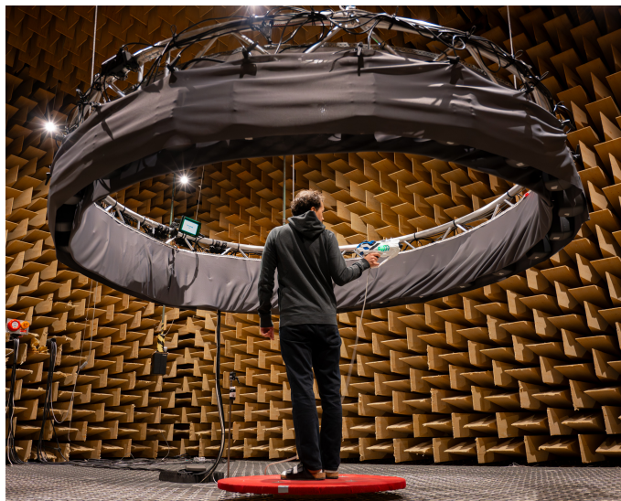
Figure 4.18: Circular loudspeaker array setup in anechoic chamber.
