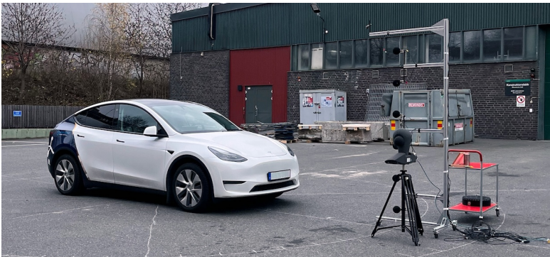
Figure 4.8: AVAS directivity measurement setup.
