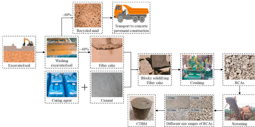
Figure 4-10. The main process of recycling filter cake to produce RCAs, from (Xu et al., 2022)
