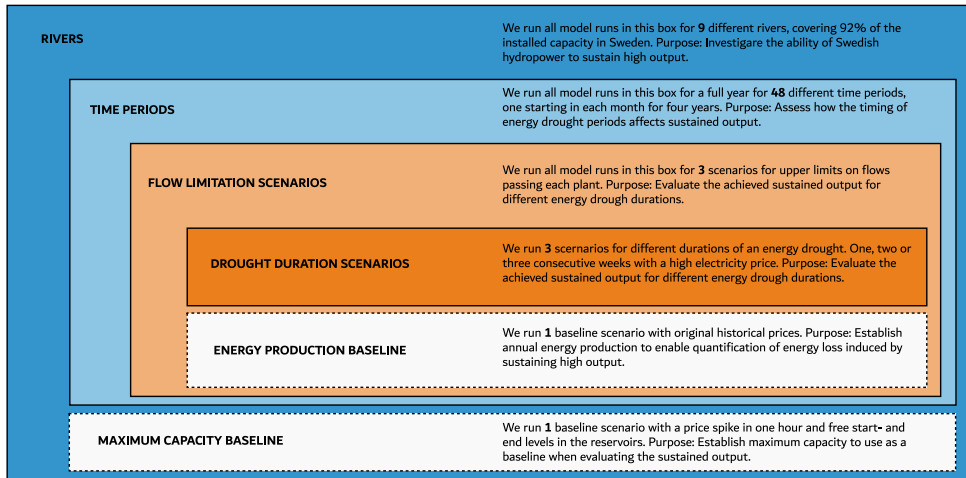
Fig. 5. A summary of all the model runs conducted in this study. The innermost box represents 3 Drought duration scenarios (one, two and three weeks; dark orange), each applied under 3 Flow limitation scenarios— Present Regime , Reduced Bottlenecks , and Unrestricted (light orange). These scenarios were tested across 48 time periods (12 months \times 4 years; light blue) for 9 different rivers (dark blue). Baseline runs, conducted to establish reference points for annual energy production and maximum capacity, are visualised in white dashed boxes. In total, this results in over 5000 model runs.
