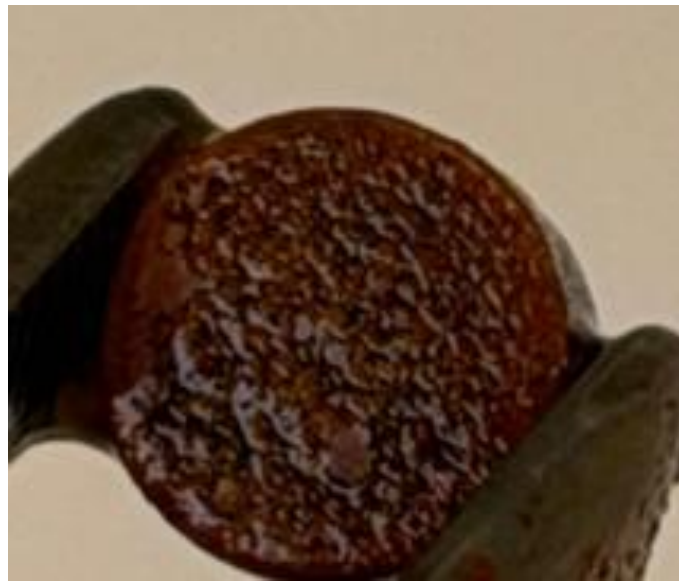
Figure 35. Visual inspection of the corroded MOX pellet and leached chukanovite when extracted from the autoclave at the end of the experiment.
