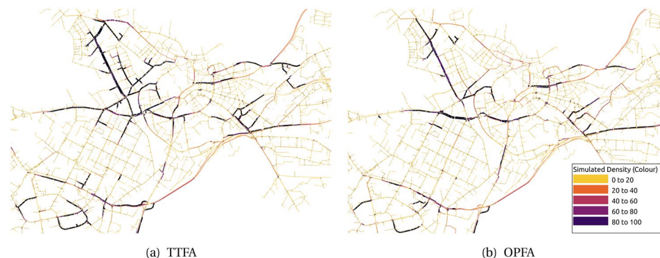
Fig. 6 Density values [veh/km] for each section in TTFA and OPFA at 9:30 in the morning peak scenario
