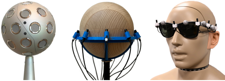
Figure 1.1: Microphone arrays suitable to capture SRIRs. From left to right: a spherical microphone array (Eigenmike EM32), an equatorial microphone array, and a head-worn microphone array on a pair of sunglasses (worn by an artificial head).
