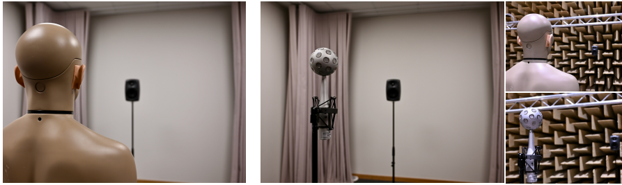
Figure 2.1: Virtual acoustic rendering can be achieved with a BRIR, for example obtained with a HATS (left). A more flexible approach uses an SRIR captured with a microphone array (center). The renderer then transforms the SRIR into a corresponding BRIR for any listener and arbitrary head rotation, provided that a set of anechoic HRIRs of that listener (top right) and anechoic array transfer functions (ATFs) (bottom right) are available.
