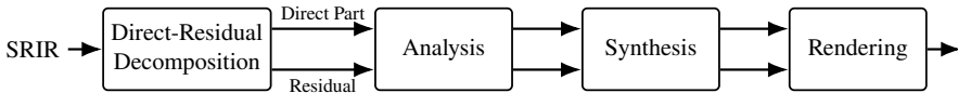
Figure 4.2: Parametric SRIR processing commonly includes a decomposition into direct and residual components and subsequent individual analysis, synthesis, and rendering of both components.
