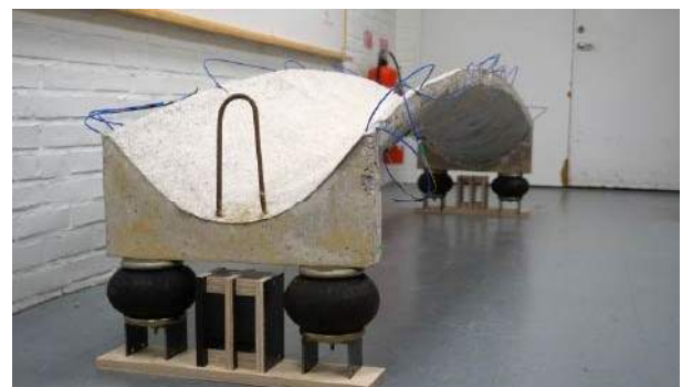
Figure 3. Specimen with two air springs under each of its abutments.
