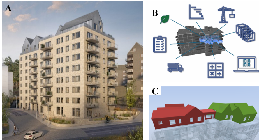
Figure 7. (A): The project case 1, Hovås Tak (Nordr, 2022), (B) Illustrating the common denominator providing interoperability opportunities between disciplines (C): The rooftop penthouses 1 and 2, coloured for sequencing according to production zones.
