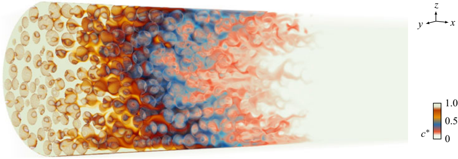
Figure 6. Snapshot of scalar transport in an inert porous reactor ( R/d = 4.7 ). The dimensionless concentration c^*(\mathbf{x}, t) = c(\mathbf{x}, t)/c_0 is injected at the left boundary at constant concentration c_0 . Filaments (or sheets) of concentration are visible near the mean front position c^* \approx 0.5 (blue region).
