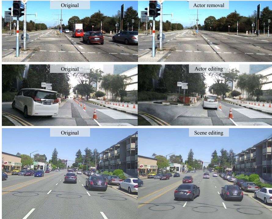
Figure 4.1: Trajectory editing through explicit scene decomposition. Three scenes reconstructed with NeuRAD [7], showing original sensor data (left) alongside renders with edited actor trajectories (right). Because each actor is represented in a canonical frame and transformed into the world via a per-timestamp pose, recorded trajectories can be replaced with arbitrary ones, enabling counterfactual scenarios.
