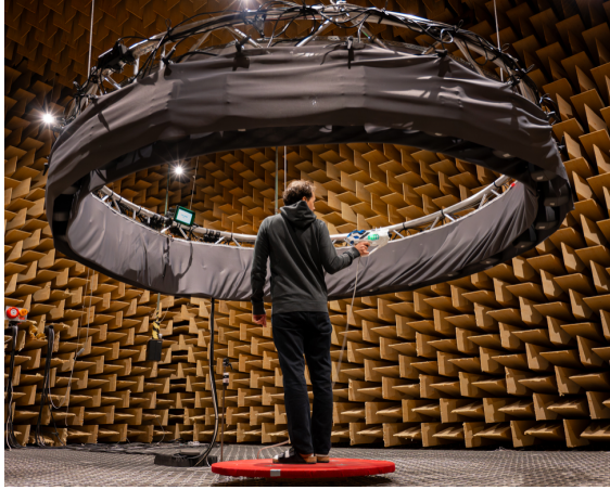
Figure 1: Participant performing the localization experiment, placed in a circular array of 24 hidden loudspeakers, indicating the perceived direction with a motion controller.
