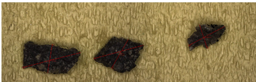
Fig. 3 Picture of three char particles and the lines representing the measure of length and width
