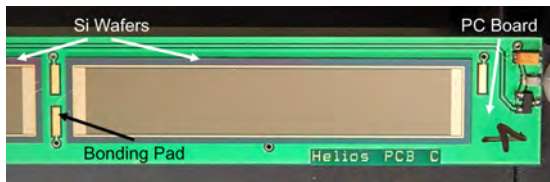
Figure 2.9: One Si PSD from the HELIOS Si array. There are electrical contacts at both short edges of the front face of each PSD (the lighter-colour part of a PSD) as well as one full-area contact at the back face. Figure from Ref. [20].
