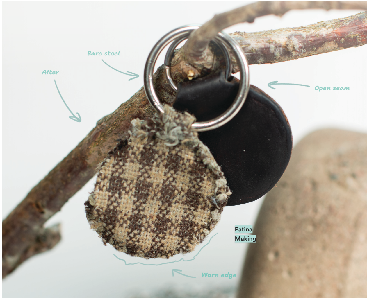
Figure 19. Bioplastic and leather tags. This image shows the tags post-use, accruing patina and eventually breaking altogether.
