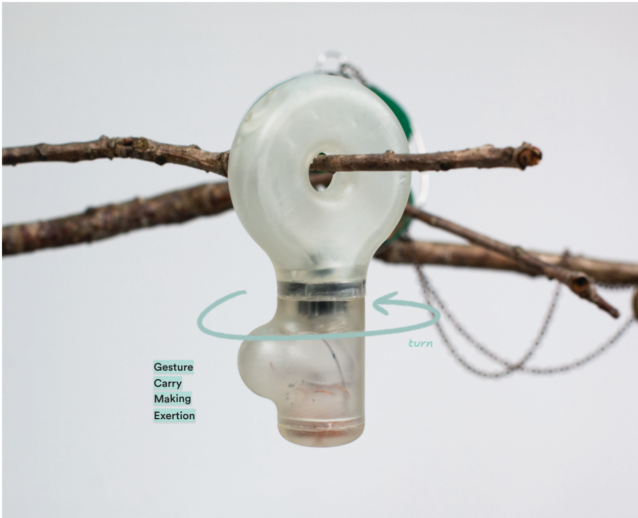
Figure 11. Product Key. This key, inspired by late 90's product design, is a device that can hold several stored RFID-keys, and allow the holder to activate and switch between them by turning the top.
