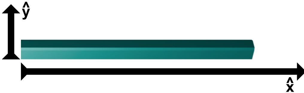
Figure 2.7: Schematic of the hybrid nanowire platform. The orientation of the nanowire ( \hat{x} ) and the resulting Rashba field ( \hat{y} ) establish the basis for the asymmetric dispersion relations ( B \parallel B_{SO} ) and topological gap opening ( B \perp B_{SO} ) discussed in Sec. 2.2.1. Note that the effective Rashba field is assumed to be oriented along \hat{y} (perpendicular to the NW) for simplicity's sake; as discussed in Paper III, this orientation is not necessarily reflected in realistic devices.
