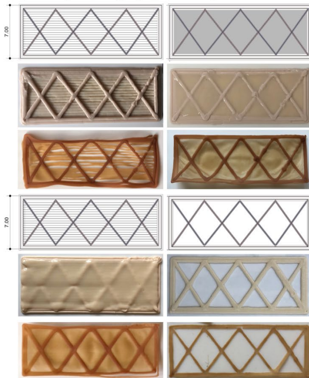
Figure 11. Toolpath design and scale transition illustrated through four phases of the research, from manual 2x2 cm extrusion tests (Phase 1) to bioprinted 5x5 cm and 7x7 cm pattern studies (Phase 2), robotically fabricated 7x20 cm patterned and layered constructs (Phase 3), to full-scale 50x20 cm solid and lattice tile demonstrations (Phase 4). The progress highlights how material behaviour is evaluated through patterning logic and deposition strategies to inform potential architectural applications.
