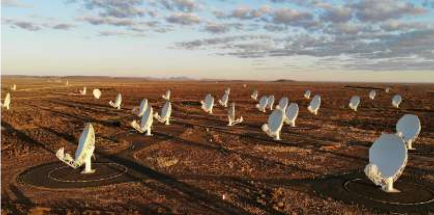
Figure 5.1: The MeerKAT radio interferometer located in the Karoo region of South Africa. The array consists of 64 dishes distributed over baselines of up to \sim 8 km.
