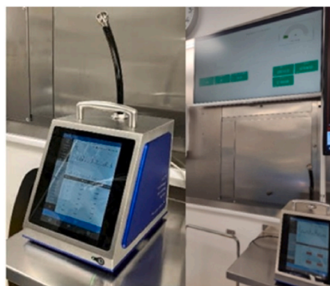
Fig. 2. Bio Aerosol Measuring System (BAMS, Zecon AB) and the screen installed on the wall of the operating room.
