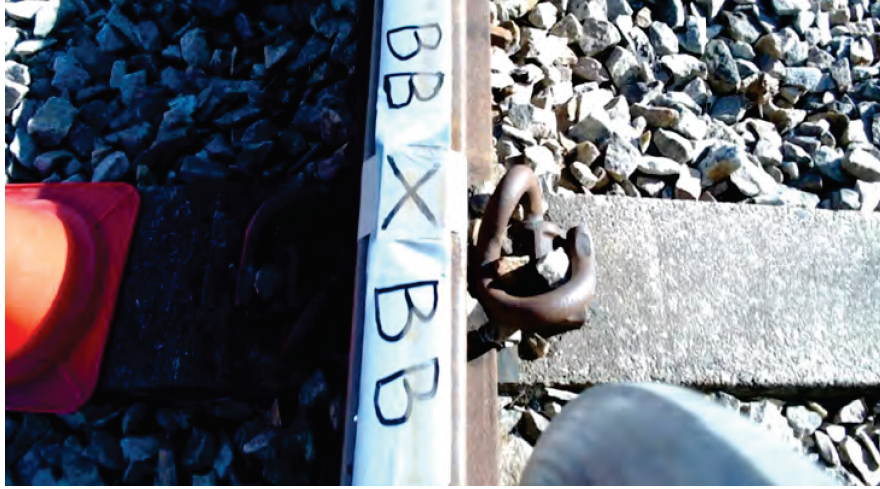
Figure 5.5: Image of simulated fault B (metal plate taped to the rail), taken in real-time by the onboard track camera.
