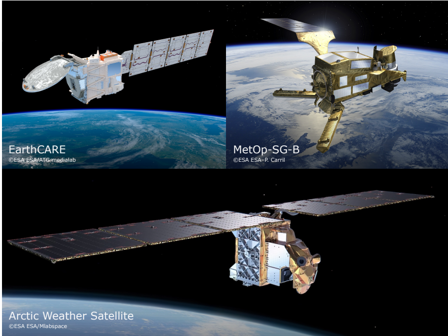
Figure 1.5: Satellites featuring in this thesis that can be used for atmospheric ice mass retrievals. EarthCARE (the successor to CloudSat) carries, among others, a cloud profiling radar and a lidar, two active instruments. The Arctic Weather Satellite carries a passive radiometer with channels between 50 and 325 GHz. The MetOp-SG-B satellites carry the Ice Cloud Imager, a passive radiometer with channels between 183 and 664 GHz.
