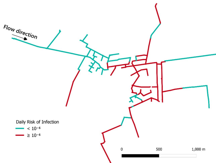
Fig. 5. Map of the WDN showing pipe segments with a daily risk of infection above 10^{-6} in red.
