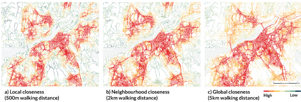
Figure 4. Closeness centrality in Gothenburg, Sweden, measured at local (a), neighbourhood (b), and city (c) scales. Image credits: Spatial Morphology Group, Chalmers University of Technology.
