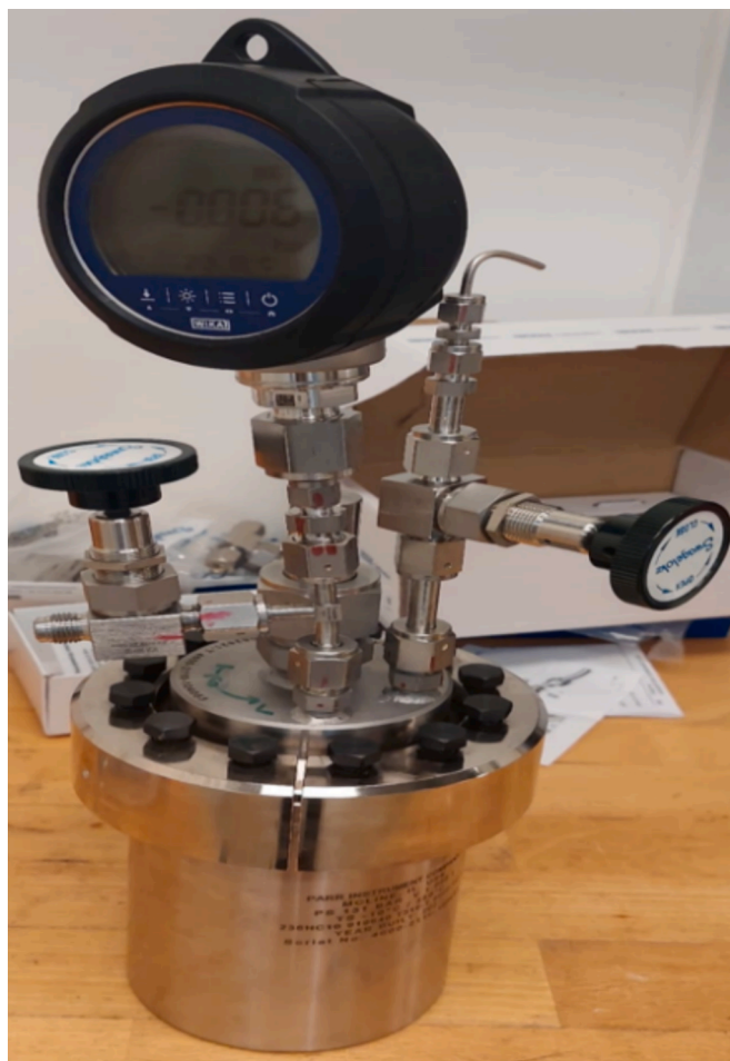
Fig. 1. Image of the autoclave used for the leaching test.
