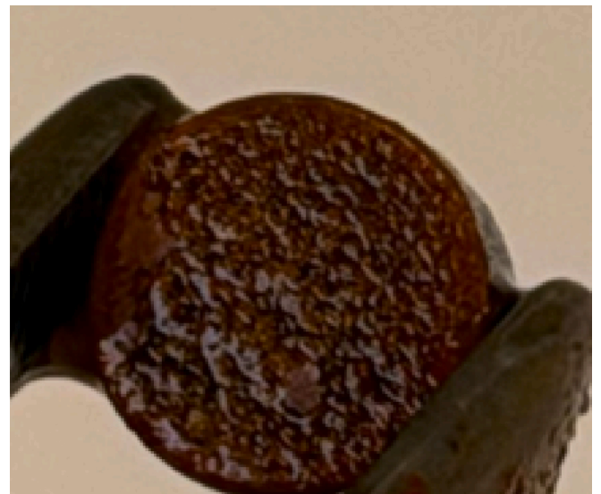
Fig. 9. Visual inspection of the corroded MOX pellet in the presence of chukanovite when extracted from the autoclave. The diameter of the MOX pellet is 8.1 mm.
