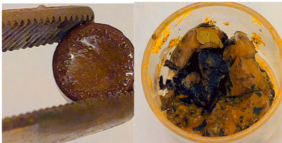
Fig. 14. Visual inspection of the corroded MOX pellet (left) and leached U-contaminated chukanovite (right) when extracted from the autoclave at the end of the experiment. The diameter of the MOX pellet and the beaker is the same as in Fig. 4.
