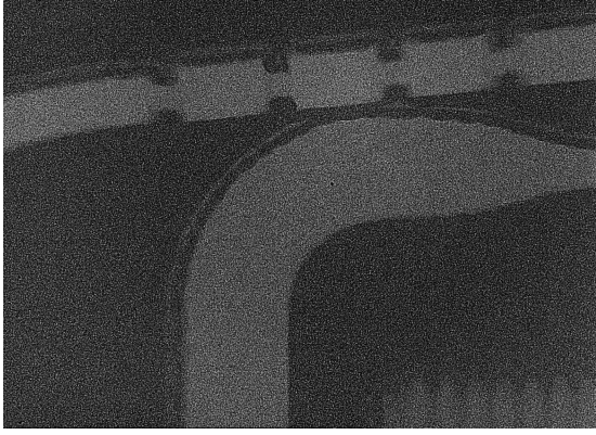
Fig. 5. X-ray image of a manufactured prototype for an old design, depicting artifacts close to the RWG channels. Due to these artifacts, the preferred minimum resolution was increased from 100 to 200 \mu\text{m} .
