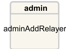
Fig. 4. A straightforward role-based access control in the DCR model for adminAddRelayer , requiring the admin role.
