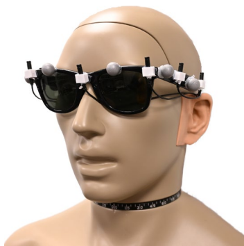
Fig. 3 Microphone array prototype with seven microphones and six tracking markers on sunglasses
