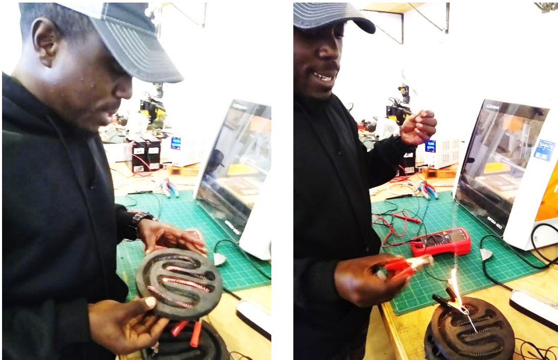
Figure 1: Photos of Leandre Niyigaba immediately after he developed an alternative means of configuring a DC-powered electric hotplate using available materials. Photos taken by Sam Unsworth, reproduced with permission.
