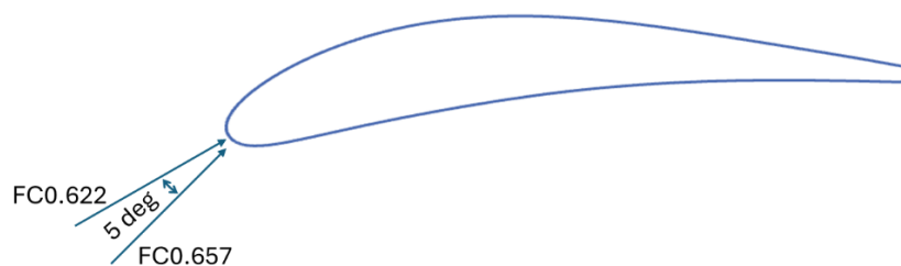
Figure 3-5 Schematic showing change in incidence angle due to flow coefficient
