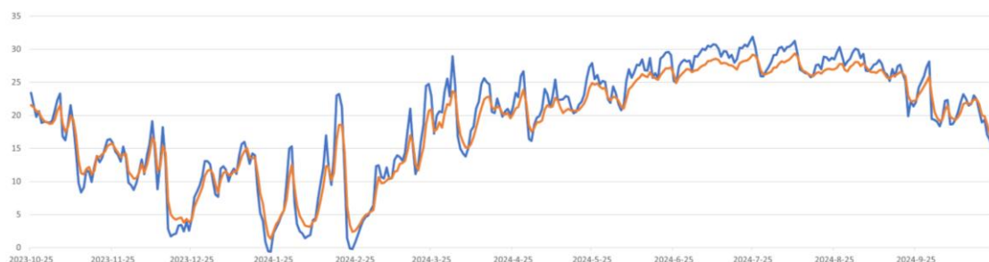
Figure 4. Comparison of average daily indoor (orange line, °C) and outdoor (blue line, °C) temperatures in the rammed earth house. No active heating or cooling equipment was used during the monitoring period, allowing the data to reflect the building's passive thermal regulation performance.
