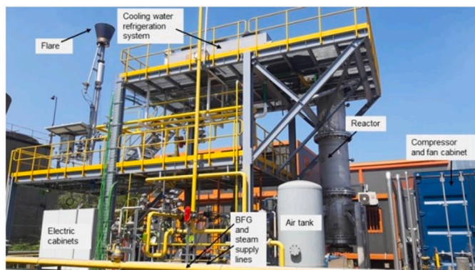
Fig. 13. Photograph of the CASOH pilot plant at ArcelorMittal Gas Lab. This plant uses sorption-enhanced water gas shift (SEWGS) to produce H_2 and decarbonize blast furnace gas (BFG) for the production of steel. Reproduced from Fernández et al. (2025), licensed under CC BY 4.0.
