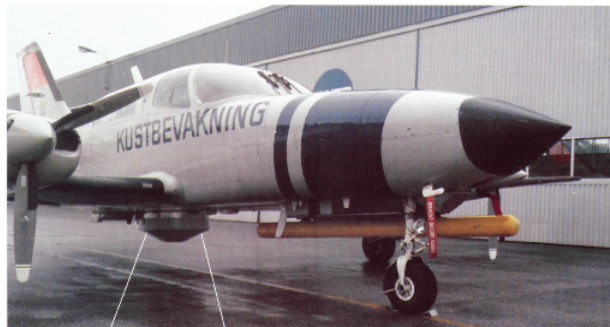
Aircraft with complete Maritime Surveillance System including Microwave Radiometer. The rotating platform with four antennas.
