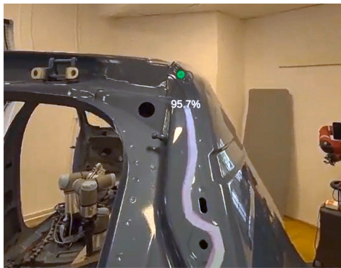
Fig. 5. Point-of-view from the trainee showing the scoring of the applied sealant.
