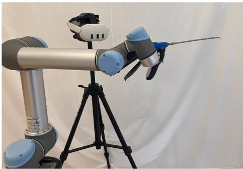
Fig. 8. Setup of the study using the UR3 and the Meta Quest 3.
