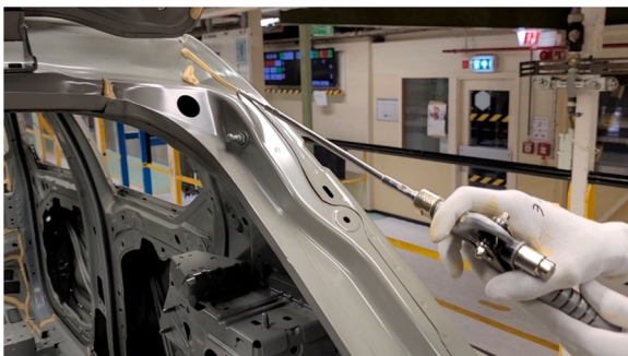
Fig. 3. Operator applying sealant to the D-pillar of a car body.
