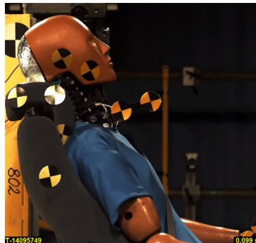
Supplementary Figure 4. Photos pre-test (T=0) and at the maximum seatback angle for the BioRID II at three different HR positions (low, mid, top).
