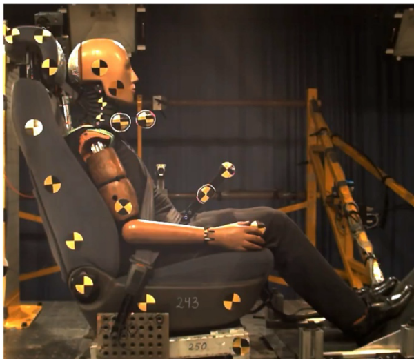
Figure 1. Test setup for (A) the prototype BioRID P50F_V2 and (B) the male BioRID II, both seated in the Saab 9-3 seat with the HR in the top position. Photos: Autoliv Sweden.
