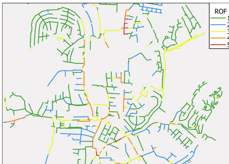
Fig. 4 GIS representation of a subset of the risk categorisation of wastewater pipes. A colour version of the figure is available in the online version of this paper
