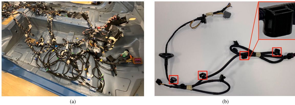
Fig. 1. (a) Example bundle of wire harnesses designed for installation on a car chassis. (b) Section of automotive wire harnesses, with clamps highlighted by red rectangles.
