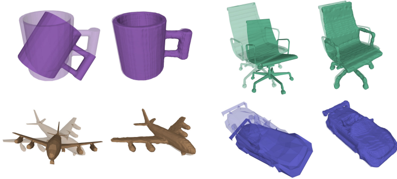
Figure 3: Example shape alignment results. The meshes on their canonical poses are shaded. Reconstructed meshes are on the right, given perturbed meshes are on the left. Post-training, shapes are aligned very closely to their canonical poses.
