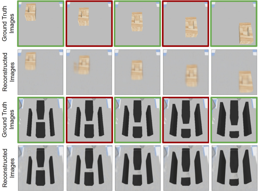
Figure 5: Comparison between reconstructed images and ground-truth images. Images with a red border are not seen during the training. However, the scene neural field can smoothly interpolate between the images seen in training and can reconstruct the unseen ones.
