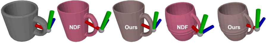
Figure 4: Comparison of resulting grasp poses. The anchor mug with expert grasp pose is shown with the gray mesh on the left. Grasp poses, represented as fingertip frames, predicted by NDF and our method are shown on the pink and the brown meshes.
