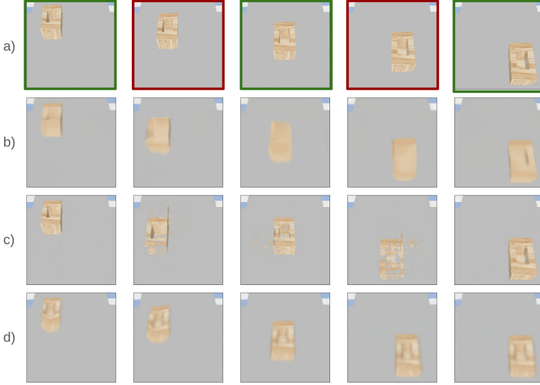
Figure 4.2: Effect of positional encoding and the deformation-based formulation on image reconstruction. Ground truth training images are marked with a green border, and unseen ones are marked with a red border in row a). Row b) and c) show the reconstructed images using neural fields with low- and high-frequency positional encodings, respectively. Row d) shows the images reconstructed using low-frequency deformation field and high-frequency template fields.
