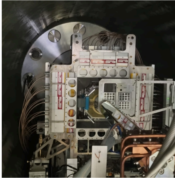
Figure 3.18: Photograph of the experimental setup installed inside the solenoidal magnet. In the foreground, the Si array is visible, followed along the beam line by the target support structure, the box-like CeBr 3 scintillation array, the LUME detectors, and the \Delta E layer of the fission-fragment detector mounted on the yellow PCB board. The beam diagnostics detectors, mounted at the end of the setup, are not visible in this photograph. The beam enters from the lower right.
