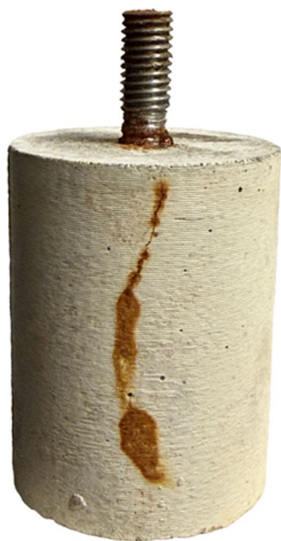
Fig. 8 Final state of specimen L-LC 3 -4 after the corrosion experiment, showing corrosion products emerging through a radial crack that reached the side of the specimen
