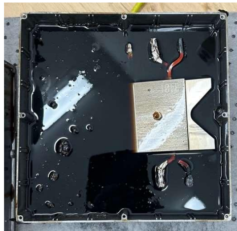
Figure 11. Degraded oil in the container with formette assembly after ageing for 288h at 180C.
