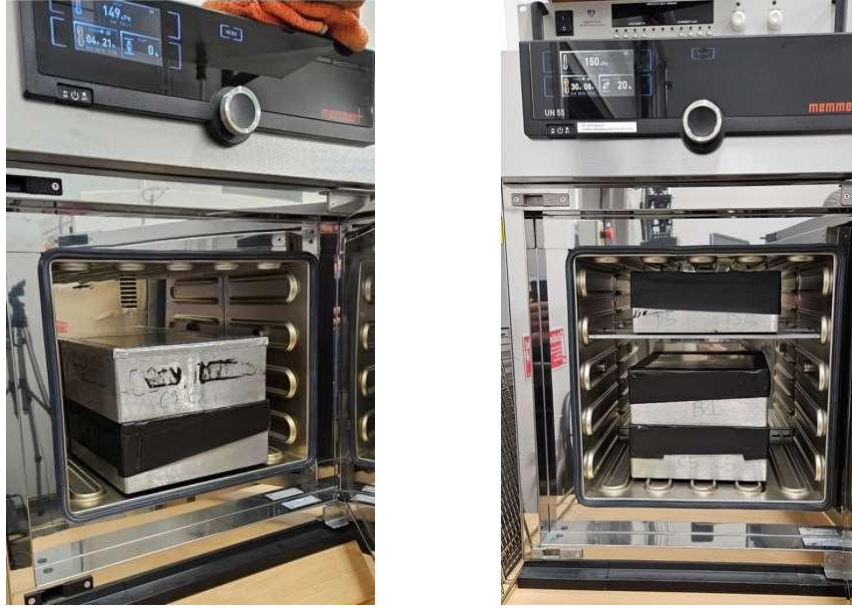
Figure 3. Containers with formettes immersed in oil inside the ovens.
