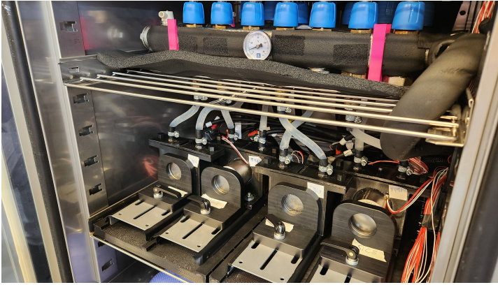
Figure 3.1: Environmental chamber setup used to control the ambient air temperature during cycling while applying localised cooling to the cell surface.
