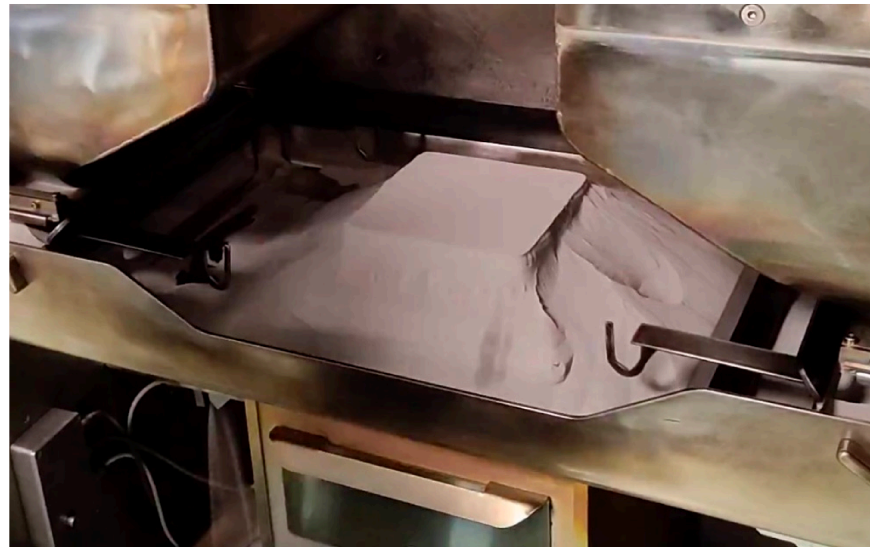
Figure 8. Build chamber with the powder cake obtained after the third build.
