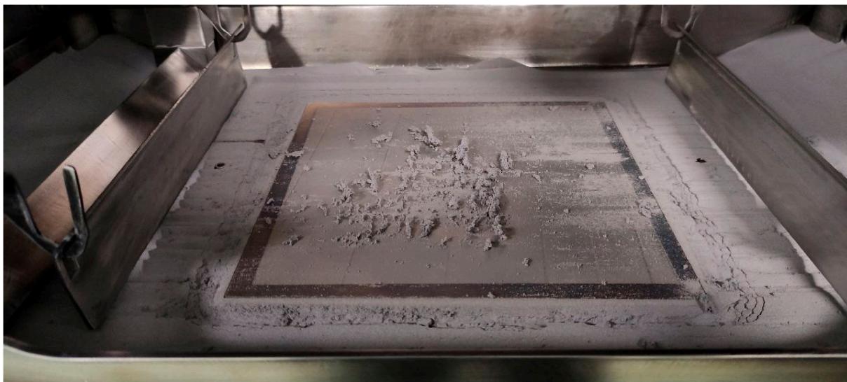
Figure 6. Build chamber with the deposited powder after the second build.
