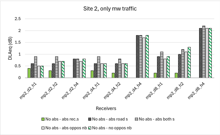
Figure 4.8: Site 2, the difference in noise reduction DL_{eq} (dB) between situation without absorbers and with different absorber applications on the noise barriers, including the additional alternatives.
