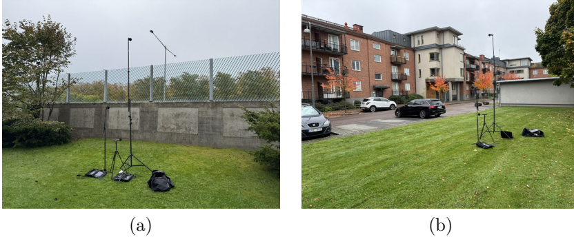
Figure 3.5: Measurement positions at Site 1 north of the motorway: (a) 4 m behind the noise barrier, (b) in the backyard 50 m from the noise barrier (photo: Akustikkonsulten).
